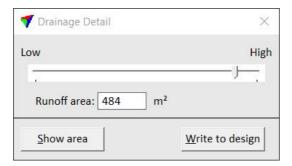
When the slider is set to **High**, the drainage display shows the paths of each single rain drop. If you move the slider closer to **Low**, the software leaves out smaller streams and only displays the major paths. The drainage network remains visible as long as you keep the **Drainage Detail** dialog open.
