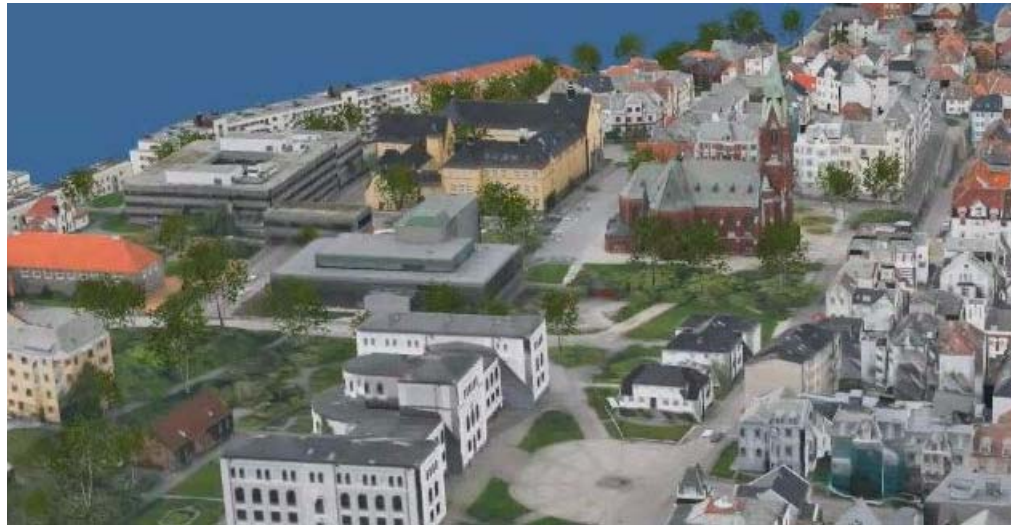
Rendered view including orthophotos draped on a DEM and building roofs, wall textures referenced on 3D building models, and RPC trees.
